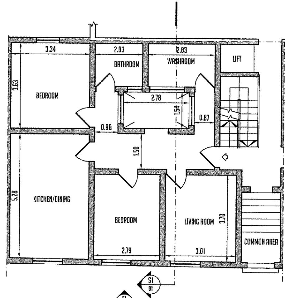
**EXISTING ELEVATED GROUND FLOOR PLAN**
